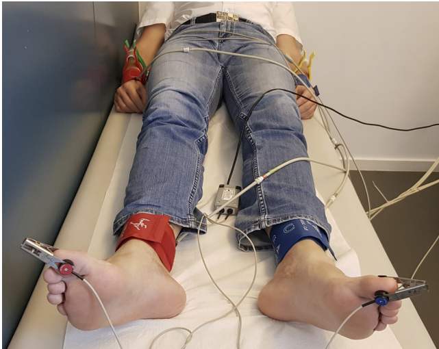
Fig. 1. Photoplethysmographic (PPG) sensors on the large toe at the foot for determination of tissue optical perfusion pressure (TOPP) and pressure cuffs at the ankle on the right (red) and left (blue) lower limb.
